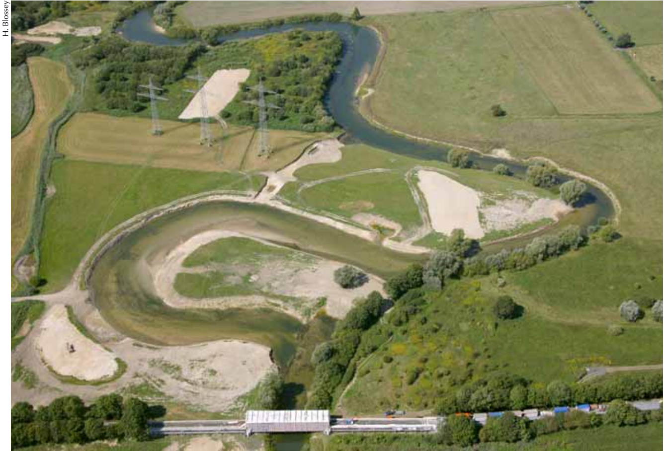
The extension of the Lippe's course in Action Block D is downriver of the bridge of the former coal mine railway in the foreground of the photo. From above it is clear that the Lippe is much wider and shallower in the new loop than it is in its old course.
