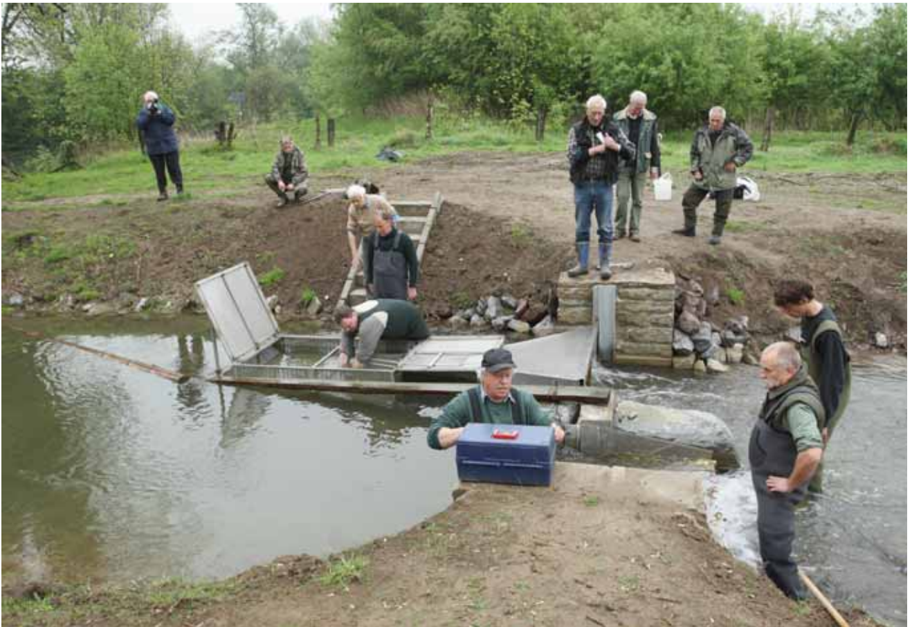
Where the bypass channel leaves the Lippe a large fish trap was installed. The migrating fish come from downriver (at right of photo) and swim into the funnel of the trap. Once a day, members of the Heessen Fishery Association count and measure the fish and then release them upstream of the trap.
