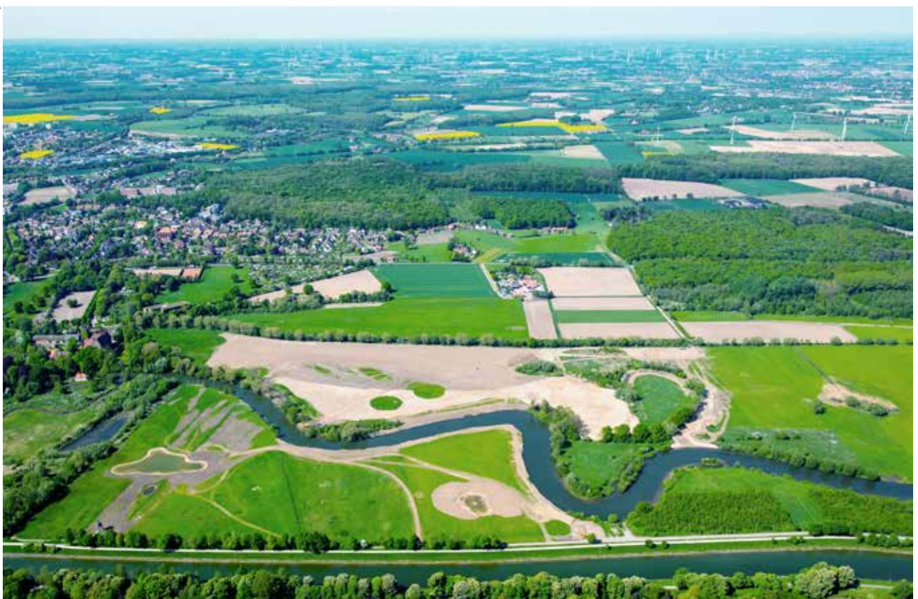
“Schlagmersch” during the restoration work: Large bodies of water and flood channels are being created, the ploughed field has become a meadow and the river bank reinforcements have been removed.
