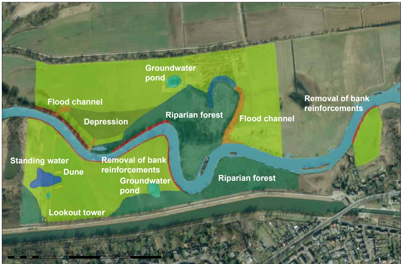
In the “Schlagmersch” project block east of Schloss Heessen the entire river bank reinforcements were removed. Flood channels connect an oxbow lake with the Lippe and permit inundation of the floodplain during highwater periods.
